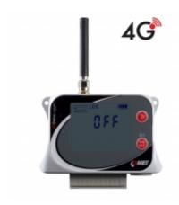
4G datalogger is designed to record from four binary inputs or from two pulse and two binary inputs. In case of exceeded set limits, SMS and JSON messages can be sent via GPRS data connection. Measured values can be sent to the internet storage <a href="COMET Cloud">COMET Cloud</a>, which is a complete monitoring, alarm and analysis system.
